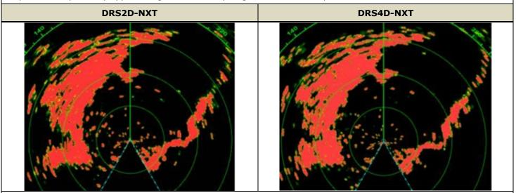
The DRS2D-NXT shows similar images to the DRS4D-NXT in a long range scale of 24 NM. Due to the longer antenna, bearing resolution is superior with the DRS4D-NXT: The DRS4D-NXT shows echoes more sharply than the DRS2D-NXT.
