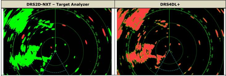
These images are from the area around the Kobe Airport in the 3 NM range scale. The DRS2D-NXT in Target Analyzer helps intuitively identify approaching and stationary targets around the airport.
