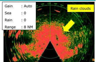
Let's see how Target Analyzer can help identify targets: After the **Target Analyzer – Rain Mode** is turned on, one approaching target in red and stationary targets in green are instantly identified under the rain shown in blue dots.
