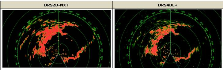
These screenshots show Osaka Bay in the 24 NM range scale. The Solid-State DRS2D-NXT is compared with the magnetron-type DRS4DL+; the DRS2D-NXT shows clearer coastlines inside Osaka Bay.
